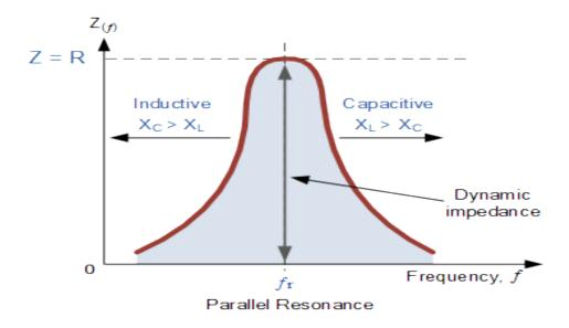
Quality Factor(Q)- It is the measure of sharpness of resonance in the circuit.
