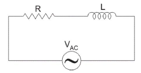
The current lags behind the voltage by a phase angle of  $\Phi$
